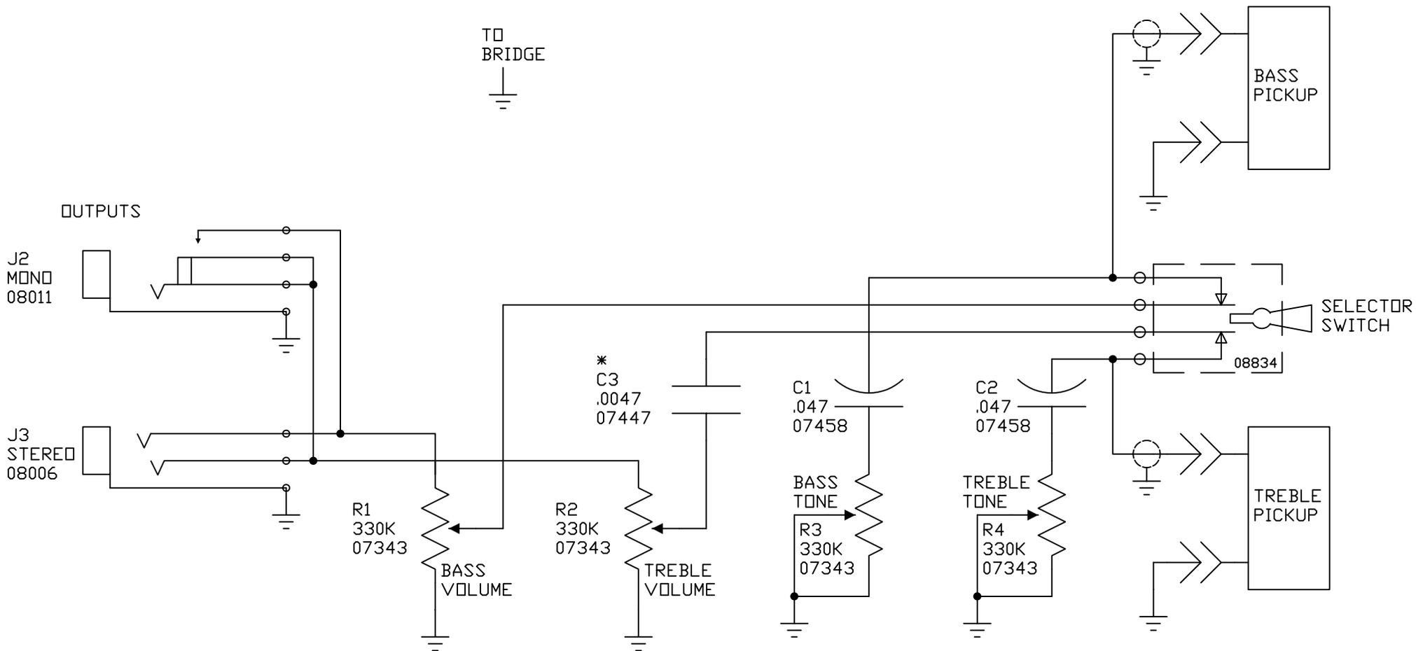
\* C3 IS REPLACED BY A SHUNT ON NEWER MODELS
